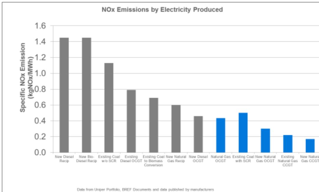
Figure 1: The NO<sub>x</sub> intensity of different technologies and fuel type
